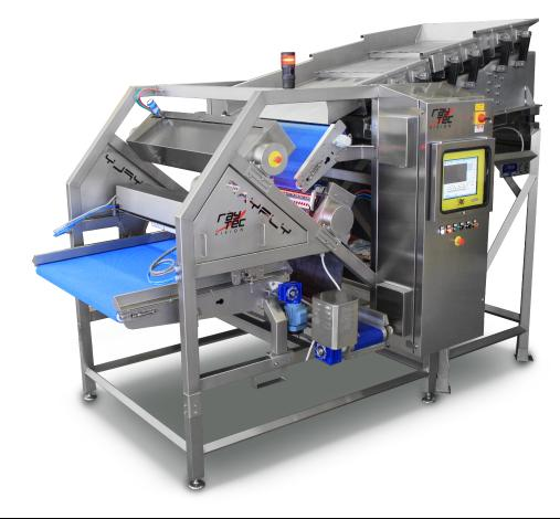
The Fototrainer technology is a combination of 4 analyses that together make the system very efficient in contaminant detection.
